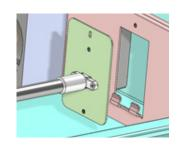
6. Connect Bulb to socket in the Bracket Assembly.
