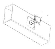
3. Remove the (2) Screws holding the NC<sup>2</sup>I Cell in place and remove the NC<sup>2</sup>I Cell from the Unit Cover.
