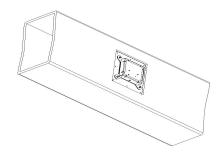
Remove the (4) Flange Nuts from the Unit Cover and Remove the Unit Cover and NCC Cell.
