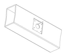
2. Drill holes around the outside edges of the previously marked hole but inside the outer holes of the Adhesive Mounting Bracket.
