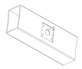
2. Drill holes around the outside edges of the previously marked hole but inside the outer holes of the Adhesive Mounting Bracket.
