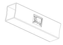
2. Remove the (4) Flange Nuts from the Unit Cover and Remove the Unit Cover and NC<sup>2</sup>I Cell.
