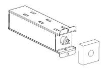
2. Exchange the Old NC<sup>2</sup>I Cell with the new NC<sup>2</sup>I Cell and replace the (2) Screws that hold it in place.
