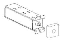
2. Exchange the Old NCC Cell with the new NCC Cell and replace the (2) Screws that hold it in place.
