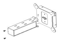
3. Replace the Cover and NC<sup>2</sup>I Cell in the duct and secure with the (4) Flange Nuts. MAKE SURE THE AIRFLOW MOVES THROUGH THE NC<sup>2</sup>I CELL (Refer to orientation and airflow above).
