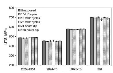
There was nominal degradation despite a higher-than-usual concentration and exposure, including no discernible differences to the surfaces of the samples.
