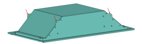
4. Hardwire CASPR BLU Tile unit into an available power source using pigtail leads and conduit connections. This is to be performed by a licensed Electrician or HVAC Installer.
