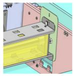
7. Attach Cell Housing to bracket with previously removed thumb screws (2).
