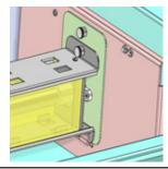
8. Install Assembly on TILE unit and secure with top thumb screw.
