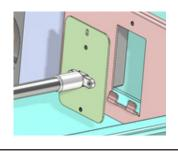
6. Connect Bulb to socket in the Bracket Assembly.
