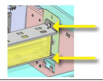
3. Remove the 2 additional screws from the Bracket Assembly.
